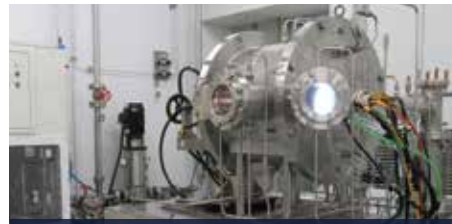
Thermal Cycling Test Apparatus of Thermal Barrier Coating (TBC)
