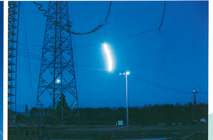
Experiment on protection of power distribution lines from lightning strokes
