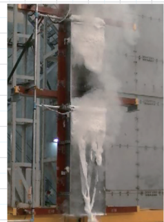
Test to verify the capabilities of the automatic fire suppression system during cable fire
