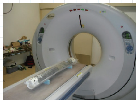
Helical X-ray CT scanner to observe boring core samples
