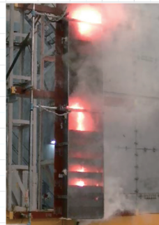
Test to verify the capabilities of the automatic fire suppression system during cable fire
