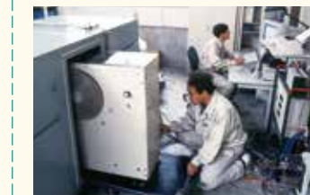
Performance evaluation testing for prototype of CO 2 heat pump
