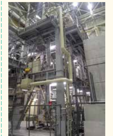
Testing facility for three-dimensional thermal hydraulics in light-water reactors
