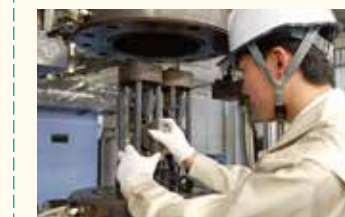
Crack propagation testing for structural materials for nuclear reactors
