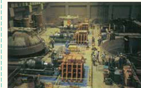
Forced vibration test inside nuclear power plant building
