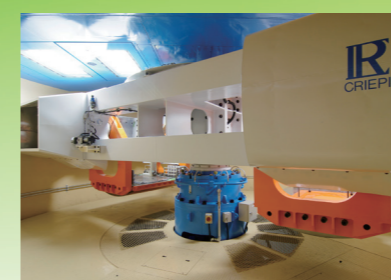
1 Geotechnical Centrifuge System
