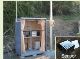
Strong-motion earthquake observation point on an outcropping rock (Ishinomaki)
