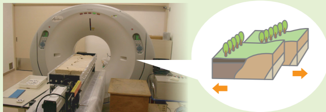
Analysis of three-dimensional fault process using a helical X-ray CT device (strike slip fault)
