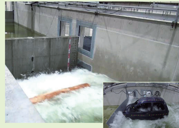
Collision experiment using flotsam
