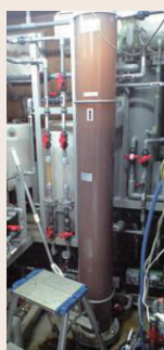
Fig. 2: Bioreactor for selenium reduction (left) and selenium treatment in on-site test at coal-fired power plant (right)
