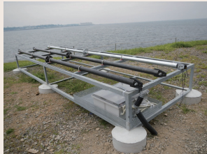
(b) Exposure test of horizontal steel pipe members (from August 2012)
