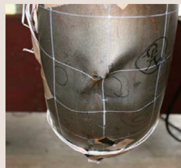
Fig. 5: Failure mode of a wall-thinning elbow under an out-of-plane bending condition by hybrid testing (Pipe size; outer diameter is 216.3 mm; wall thickness is 5.8 mm)
