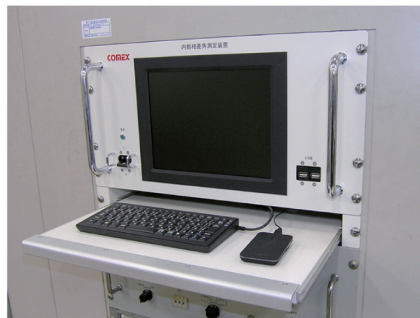
Photo 2 Rotor angle measurement equipment
