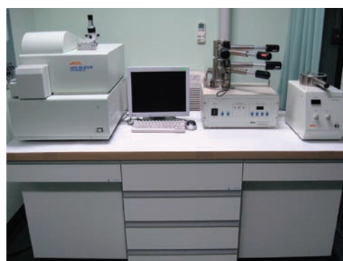
Transmission electron microscope (left) Ion slicer (center) Holder station (right) Plasma cleaner
