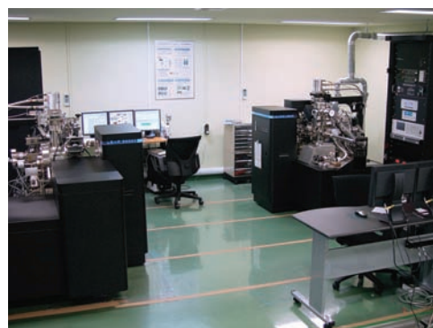
3-dimensional atom probe (left) Laser atom probe with wide-range detector (right) Atom probe with reflectron
