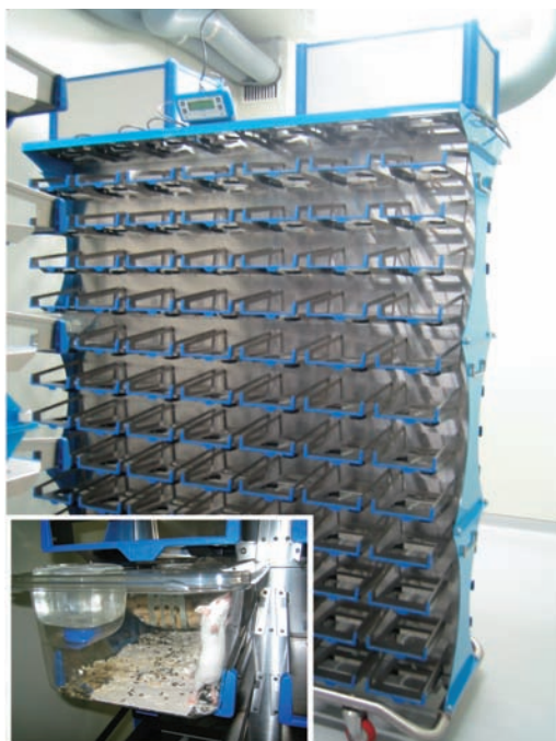
IVC racks in P2A clean breeding room
