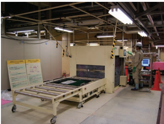
Fig.2 Verification test for surface contamination measurement at the Kashiwazaki-Kariwa Nuclear Power Station of Tokyo Electric Power Company
