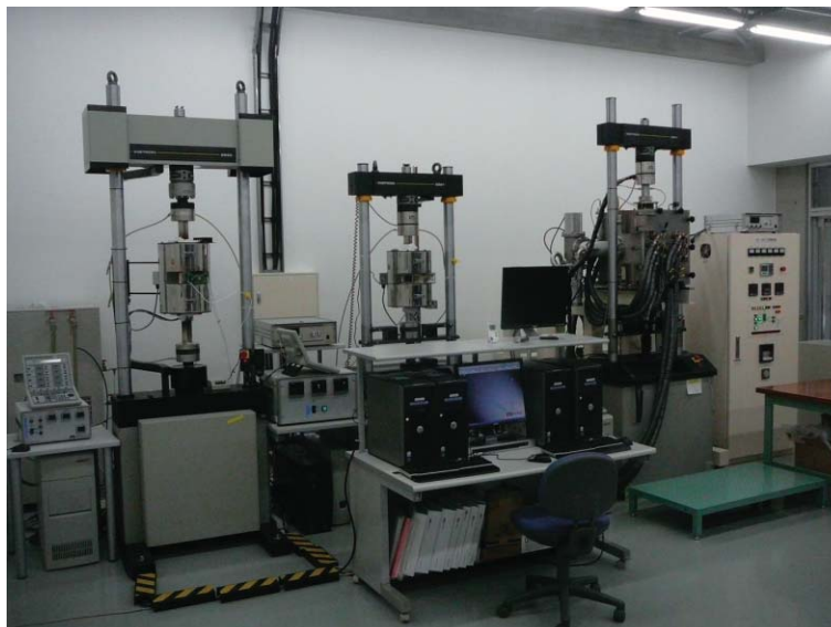
Total view of Long-term creep-fatigue test facility
