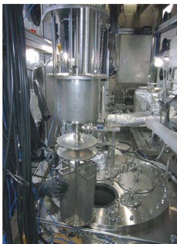
Fig.5 Photos and plain view of engineering-scale electrorefiner with liquid Cd transport to the distillator.
