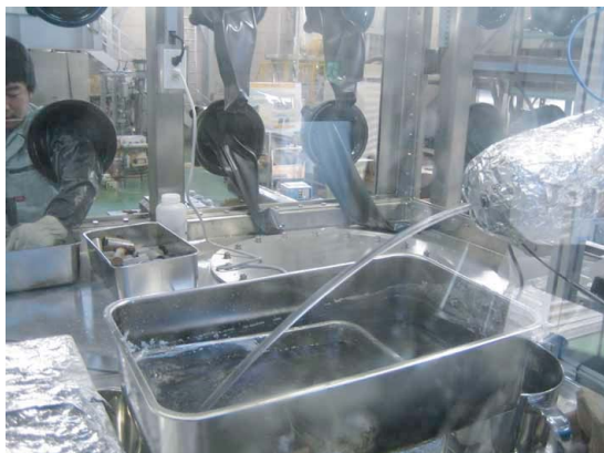
Fig. 3 Gravity transport test with molten salt.
