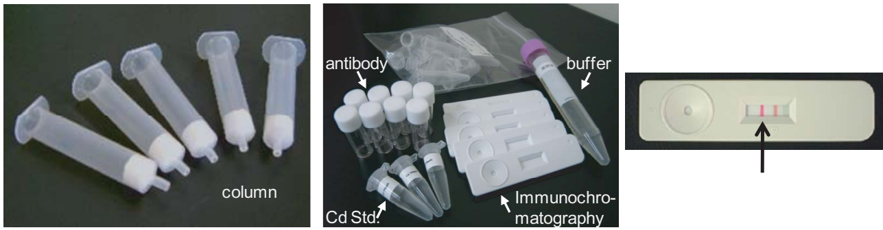
Fig.1 Contents of the cadmium test kit (left and middle) and result of the immunochromatography (right) In the right photograph, the arrow points to the red band showing concentration of cadmium.
