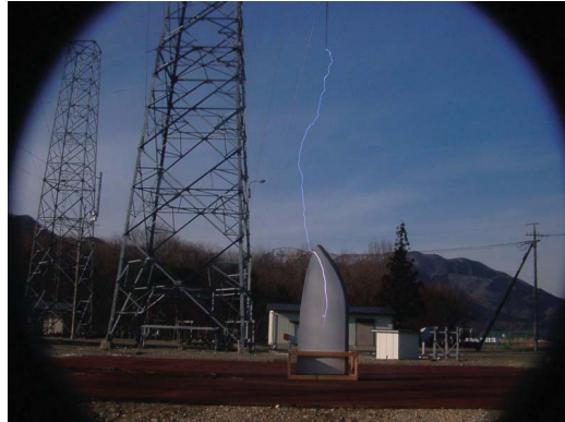
Fig.1 Large-scale thunderbolt test to a wing of wind power generator
