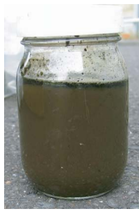
Fig.2 Water extracted from the sewage sludge.
