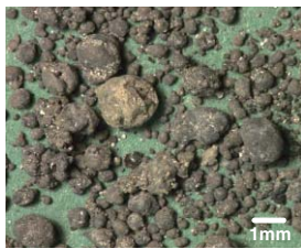
Fig.4 Heat-famed CGS example ; form rounded, produced by retining for 5-7 min. at approx. 1000°C
