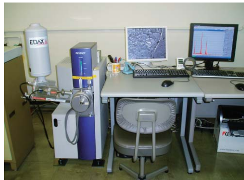
Compact-size ESEM equipped with EDS x-ray microanalyser
