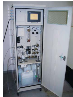
External (upper) and internal (lower) view of online boron monitor
