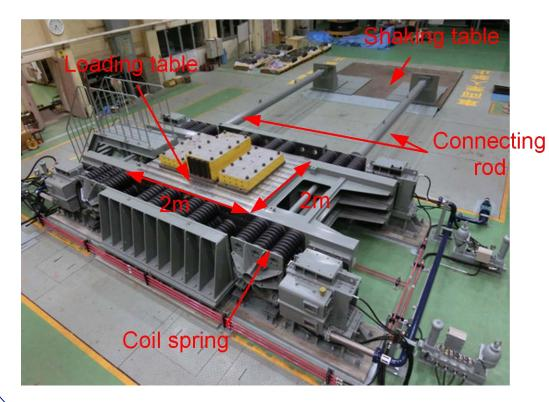
table size :2m/2m Max Load:10t Max Acc.: 20g Max Vel.: 3.14m/s Max Disp.: 0.05m Freq.:10Hz/sine curve
