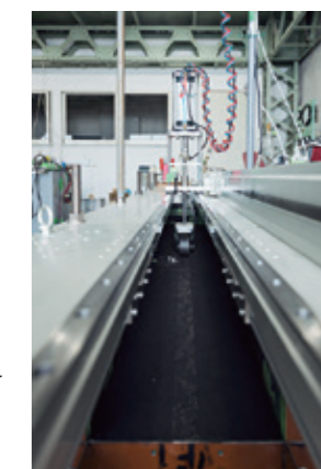
Mock tire used to run over the road surface in the small, indoor mock-up testing facility
