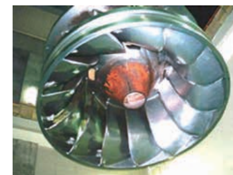
Impeller of a Francis turbine (rotating portion) (Excerpt from Kansai Electric Power's official website)
