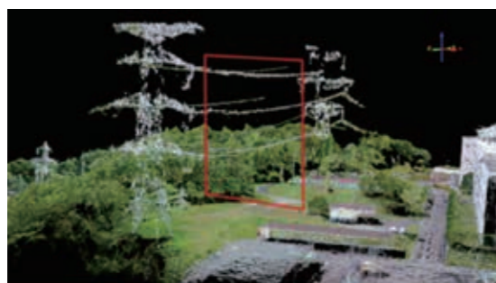
An example of utilizing drones in power line-tree distance evaluation
