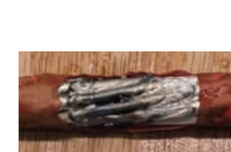
0 strands fuse (Electric charge: 491 coulombs)
