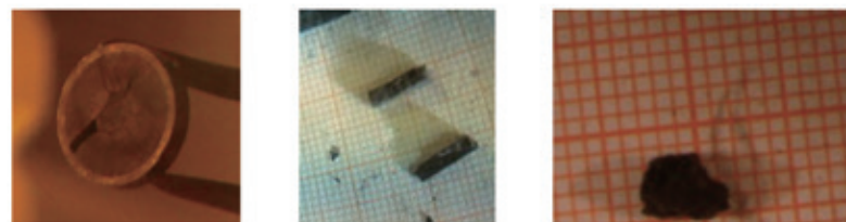
Spent fuel fragment TMI-2 (Molten pool portion) TMI-2 (Crust portion)
