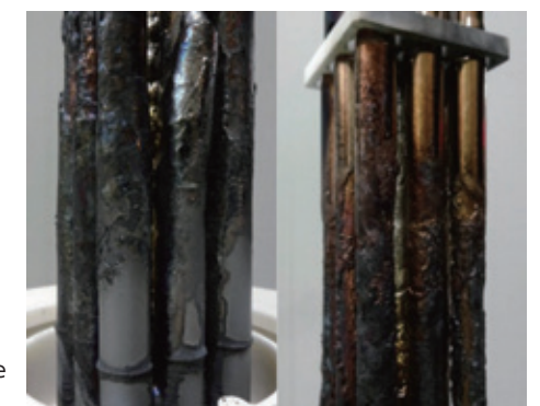
A test fuel bundle after out-of-pile severe fuel damage test in steam-limited atmosphere above 2000°C
